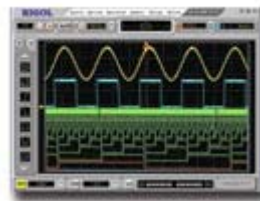
Duration Trigger: Combination of Pattern Trigger and Pulse Width Trigger
